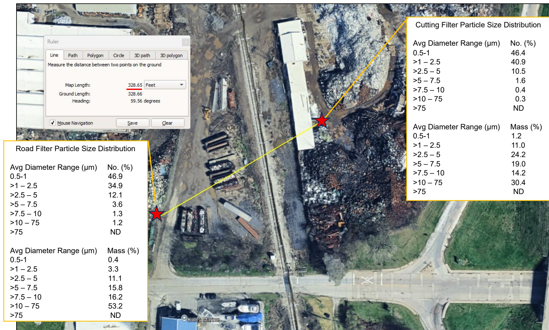
Figure 2. Road Hi-Vol Sampler and Torch Cutting Hi-Vol Sampler Particle Size Distributions (100 m apart)
